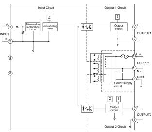
Note: Single-output models do not contain the output-2 circuit.
